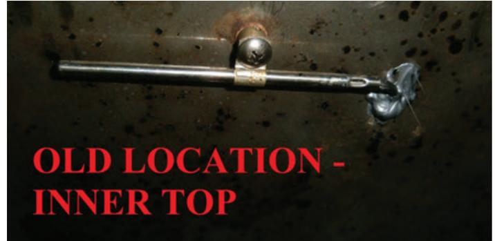
7. Replace screw back into riv-nut to fill the hole so there is no opening in the interior compartment.
